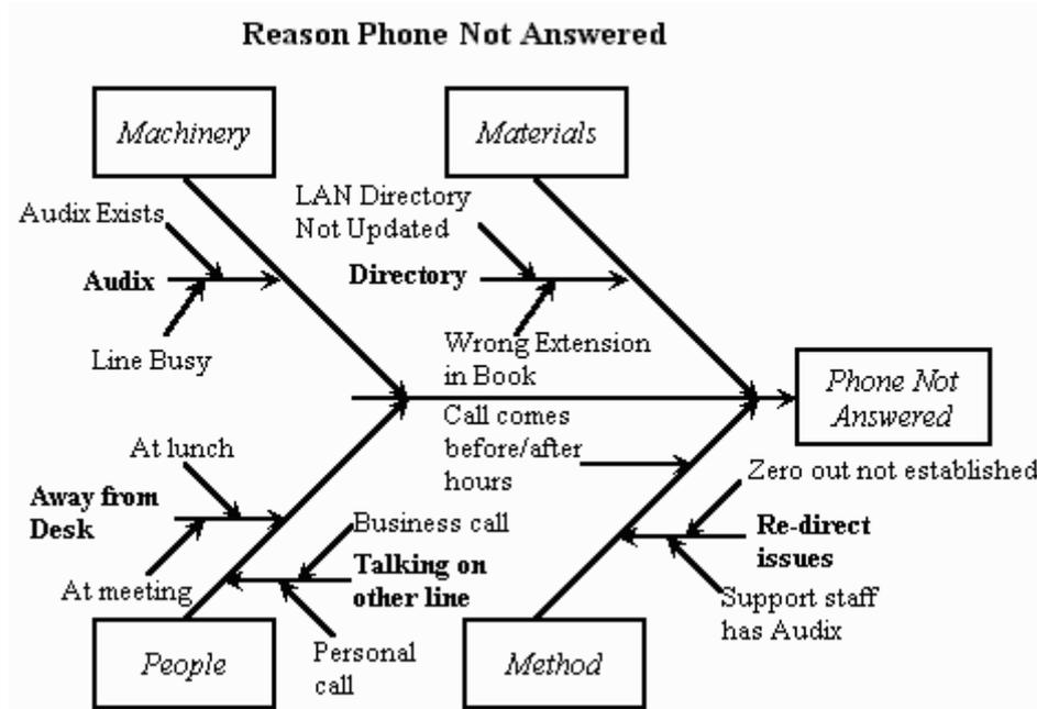
Fig.12 A Cause and Effect Diagram
