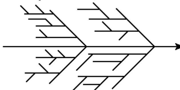
Fig.10. A Cause and Effect Diagram
